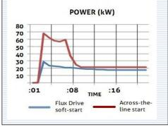
centrifugal devices, torque requirements quickly drop. This "unloads" the motor and results in lower amperage and kW consumption.
