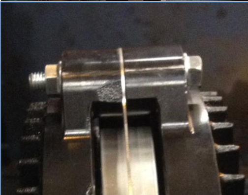
A single air gap spacer shim installed on an FSC
