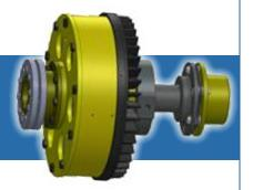
Flux Drive Inline Adjustable Speed Drive (ASD-IL) is a Soft-Start Coupling with the added ability to configure linear engagement between the rotating magnets and a patented induction rotor - thus allowing for cushioned start, vibration reduction, mis-alignment correction, variable speed control and substantial energy savings.
